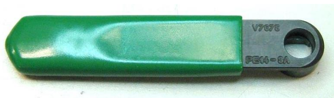
Pinion tool to unscrew the pinion.
